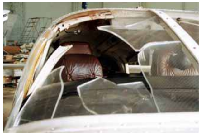
While on approach to a southern USA airport in March 2003, this PA-34 aircraft struck a pair of red-breasted mergansers at 800 feet AGL. The birds penetrated both windshields. The pilot was not hurt.
